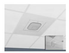
This locking 2' x 2' suspended ceiling tile enclosure is designed for APs and DAS remote units with detachable antennas. This white powder-coated steel enclosure replaces a standard ceiling tile and is UL listed for installation in the plenum space. Interchangeable doors mount leading vendors APs and antennas nearly flush to the ceiling to provide for a professional, aesthetic installation. The interchangeable doors simplify AP moves, adds, and changes without lifting ceiling tiles.
