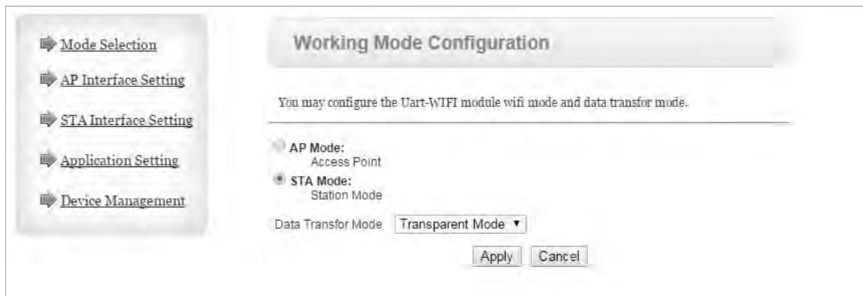
Figure 3. WiFi Interface Working Mode Configuration Web Page
