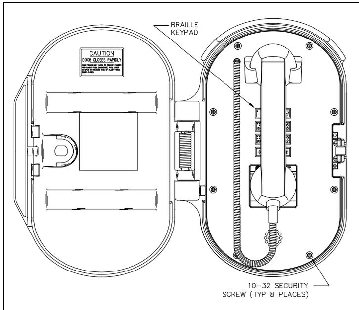
Figure 3. Model 226-001 Public Access Telephone with spring loaded door in the open position
