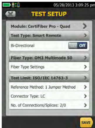
Set-up or view test limits, fiber types, and testing attributes in the field or the office.
