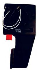
Use with an ISN-SM-50 Seismic Detector to monitor safes and strong room doors with exposed keyholes. A microswitch inside the swivel plate monitors movement. Any unauthorized swiveling movement immediately triggers an alarm. When the system is armed, the swivel plate completely covers the keyhole. When the system is disarmed, the swivel plate swings 90° away from the keyhole.
