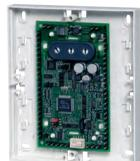
The SE 320 LSNi SmartKey arming device with connectable code keypad/reader or just with code keypad is a system solution for arming/disarming
