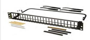
24 port unloaded flat panel for rear loading HDJ series of jacks and accessories. Includes rear management bar and straps. Occupies 1 rack unit of space, 1.75" x 19".
