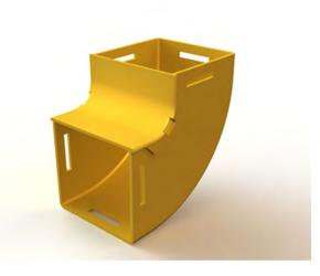
Vertical Elbows are used to connect horizontal routes at different heights or to allow the fiber path to be raised or lowered to avoid obstacles. They are available with or without covers. The retrofit versions come with split covers that are used where there is existing fiber.
