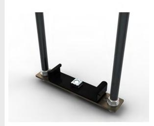
Suspension kits are used to suspend raceway from existing metal-work. Includes mounting bracket, two straight brackets, two 15" long 16mm threaded rods and hardware.
