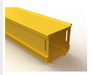
Solid duct is available with and without covers in five sizes. The unique design of the hinged cover allows it to remain in an open position while fiber is installed in the raceway. All sizes are 6' 3-3/8" long and are slotted at each end for snapping to each other or to fittings with a slotted joiner.
