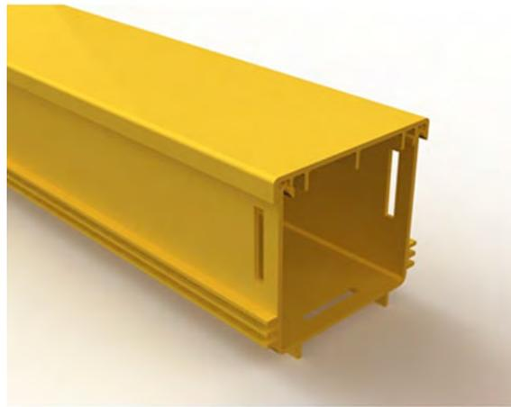
Solid duct is available with and without covers in five sizes. The unique design of the hinged cover allows it to remain in an open position while fiber is installed in the raceway. All sizes are 6' 3-3/8" long and are slotted at each end for snapping to each other or to fittings with a slotted joiner.
