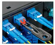
To release: Insert the removal tool, which attaches to the blockout device
