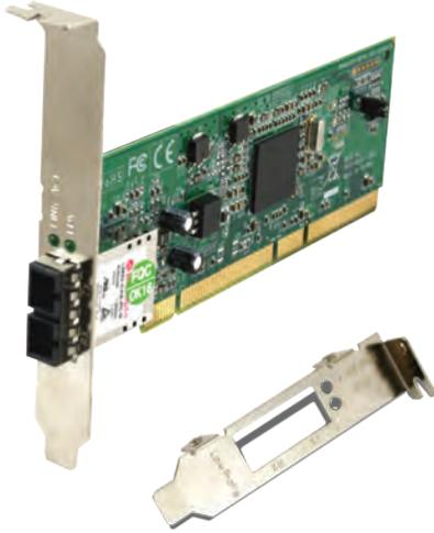
The N-GxX-xC-03 Gigabit Ethernet NIC provides a 1000Base-SX/LX fiber port, delivering fiber optic connectivity to the desktop for fiber rich LAN environments and works with both 32- and 64-bit PCI 2.2 bus slots. With both standard and low profile form factors, driver support for most common operating systems and plug-and-play capability, installation is a breeze in virtually any PC in your network.
