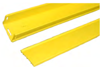
SRS-STHT-NUNU-YL-A SpeedPRO™ Straight Solid Channel with hinged cover, 100 mm x 100 mm (4 in x 4 in), 2 m (6 ft 6 in) length, yellow
