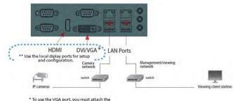
\* To use the VGA port, you must attach the provided adapter.
