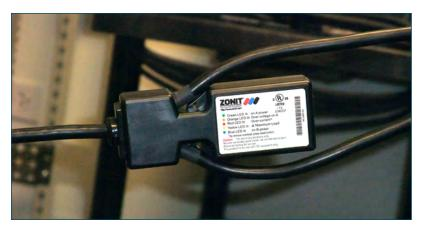
The µATS™ L-Y versions allow a single µATS™ unit to protect 2 or 3 devices from a power failure simultaneously. Please note that the total load of all served devices cannot exceed the rated load of the  $\mu ATS^{m}.$
