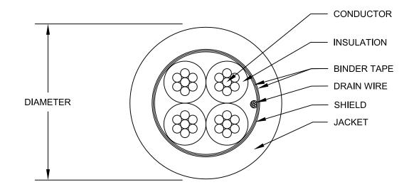
CONDUCTOR: #10AWG (7/w) Tinned Copper Class B Strand per ASTM B8, B33
