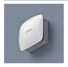
High-density WiFi installations require a large number of WAPs to be mounted throughout the facility. The Model 900 mounts and secures WAPs from many vendors directly on the wall, with a convenient location to terminate the cable. The 900 can be mounted directly over a wall outlet or anywhere on the wall or ceiling. The 900 back plate is fastened to the wall, the WAP is fastened to the 900 front plate, cabling is terminated inside, and the two halves are fastened together to form a box.
