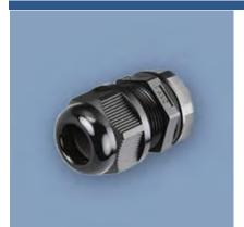
Cord Grip Connector Option - For field termination. The polyamide cable gland with split seal A-type clamping design is mounted through a knockout hole or cutout in an enclosure, and provides a watertight seal for pre-terminated Ethernet cable pass-through. The connector is strain relieving, even after tightening, and supports larger CAT 6a cable diameters.
