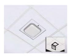
This locking retrofit door is designed to provide a convenient way to mount and secure most vendors WAPs in model 1075, 1076, 1077, and 1078 Series WAP enclosures. Simply unlock door and remove three nuts from hinge to replace door. Impact resistant, white ABS plastic dome UL classified and virtually transparent to wireless signals. Simplify equipment replacement without lifting ceiling tiles.
