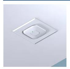
Model 1043 offers the simplest way to recess WAPs into the ceiling for an aesthetic, professional installation. A cutout is made in the ceiling and the backbox is fastened to the ceiling joists (new construction). The WAP fastens to a WAP-specific trim, and the trim to the back-box. The WAP is recessed into the ceiling much like a recessed light fixture. Access point trim can be swapped easily for new trim if the WAP brand or model changes in the future. See specs for AP-specific model names.
