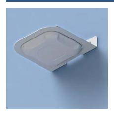
Many WAP manufacturers recommend WAPs be mounted in a horizontal orientation. Secure APs from most manufacturers in areas where wall mounting may be required, such as residence halls, hotels, and other hard lid venues. The WAP is partially recessed into the right-angle bracket, exposing only the antenna face of the AP. Conduit, raceways, and cable can be terminated in the bracket. The WAP can be locked in place using the manufacturer's locking features. Specify AP and model when ordering.
