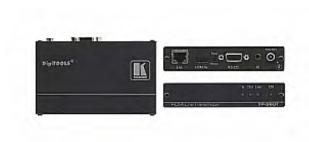
The TP-580T is a high-performance, HDBaseT twisted pair transmitter for 4K@60 UHD (4:2:0), 2Kx4K HDMI, bidirectional RS-232 and IR signals. The TP-580T inputs HDMI, RS-232, and IR signals and converts them into an HDBaseT twisted pair signal that it transmits to a TP-580R receiver.
