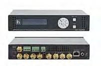
The FC-340S is a broadcast-quality video scaler and audio embedder/de-embedder for digital signals up to 3G HD-SDI. The unit inputs SDI and AES/3id signals and simultaneously outputs two SDI and composite video signals while the audio embedded in the SDI input signal is output to both AES/3id and balanced stereo audio outputs.
