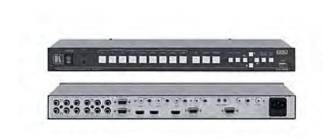
The VP-728 is a 9-input scaler/switcher for analog and digital video, unbalanced stereo, and S/PDIF audio signals. It up- or down-scales any video signal: composite, s-Video (Y/C), component video (YUV), HDMI, computer graphics video and JPEG files to a selectable graphics or HDTV output resolution via identical HDMI or 15-pin HD outputs. It provides glitch-free switching between sources through FTB™ (fade-thru-black) switching technology.
