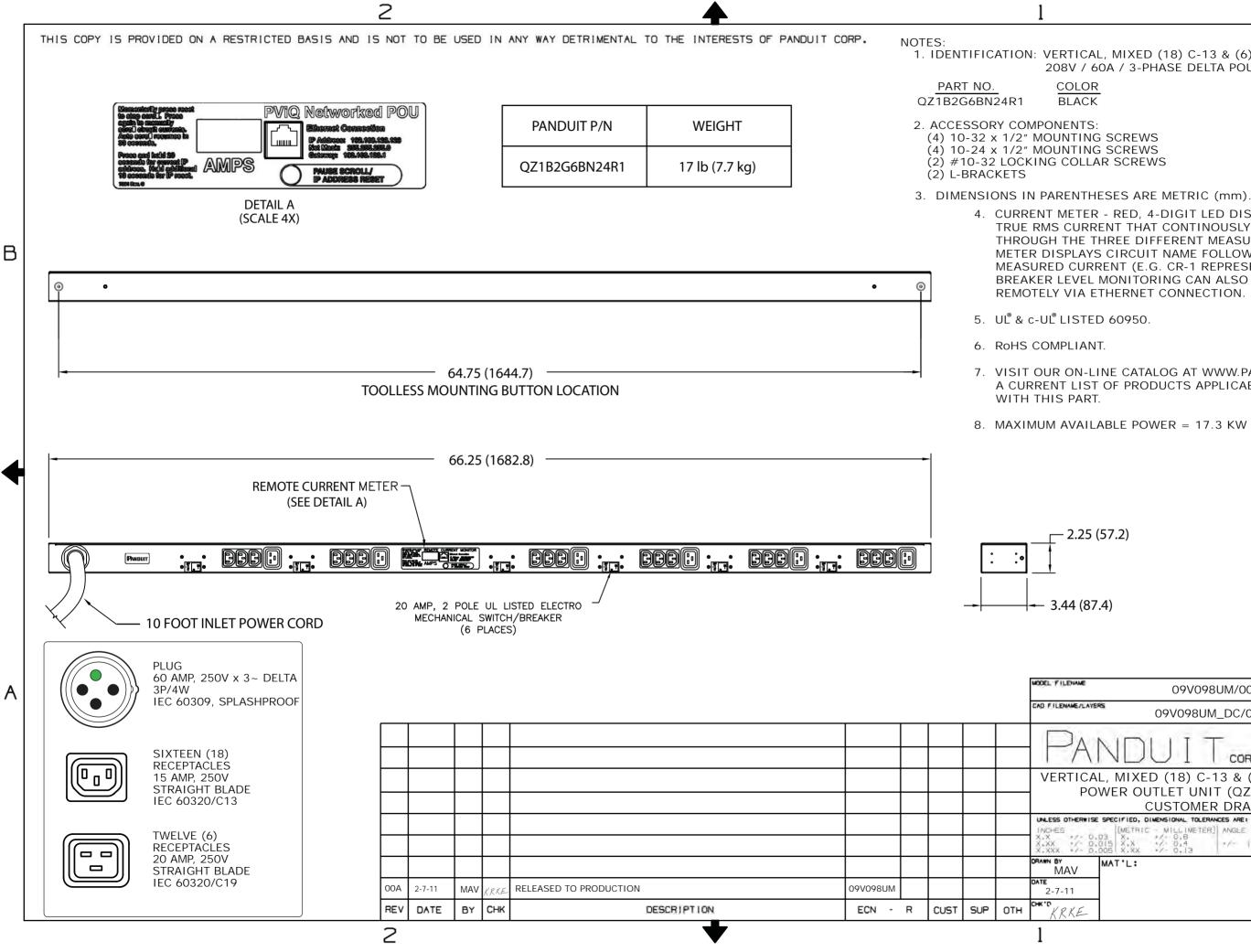
1. IDENTIFICATION: VERTICAL, MIXED (18) C-13 & (6) C-19 NETWORKED 208V / 60A / 3-PHASE DELTA POU
