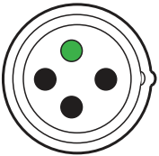
PLUG 60 AMP, 250V x 3~ DELTA 3P/4W IEC 60309, WATERTIGHT
