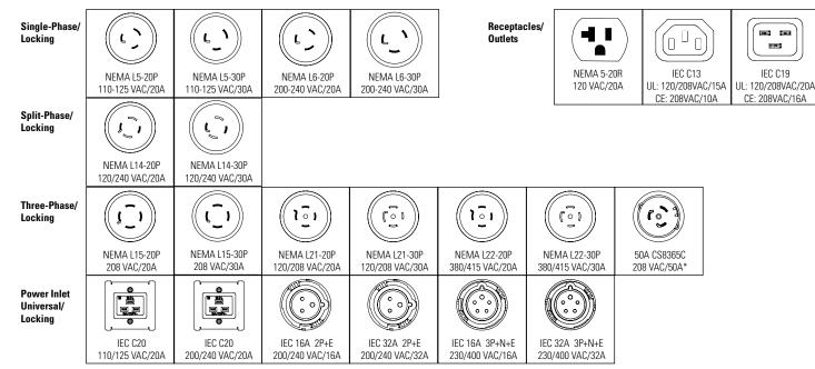
\* Note: 50A CS8365C is rated for 50A, but maximum input is 35A on three breaker PDUs.
