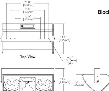
Note: FRi-2082 Loudspeaker shown. All dimensions for FRi-28LPM equal except where Ubracket is used. FRi-28LPM excludes U-bracket and mounting hardware.
