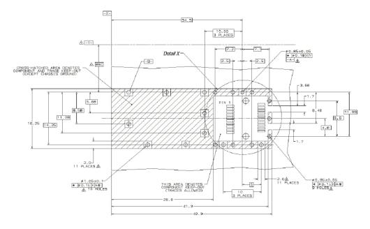
Datum and Basic Dimension Established by Customer Rads and Vias are Chassis Ground, 11 Places Chrough Holes are Unplated
