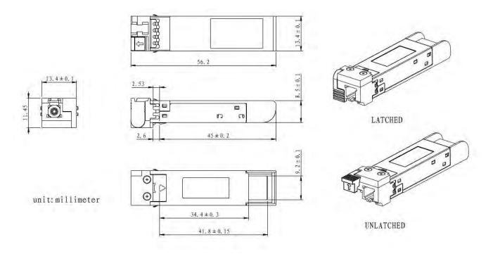
ALL DIMENSIONS ARE  $\pm 0.2 \text{mm}$  UNLESS OTHERWISE SPECIFIED UNIT: mm
