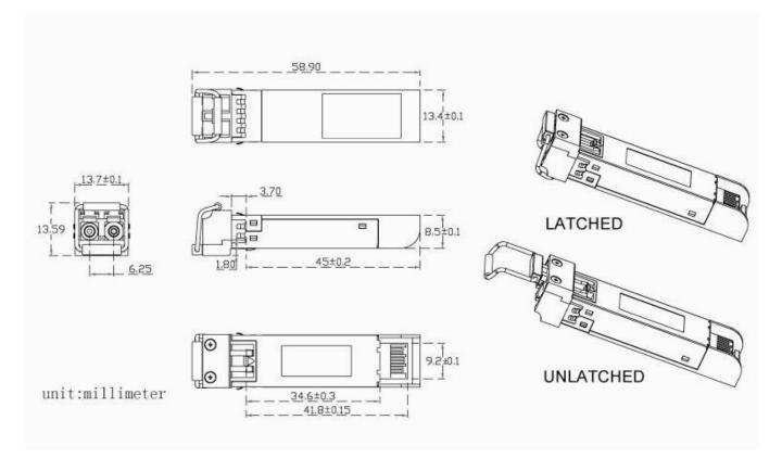
ALL DIMENSIONS ARE  $\pm 0.2 \text{mm}$  UNLESS OTHERWISE SPECIFIED UNIT: mm
