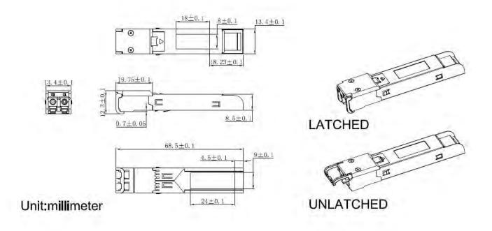
ALL DIMENSIONS ARE  $\pm 0.2 \text{mm}$  UNLESS OTHERWISE SPECIFIED UNIT: mm
