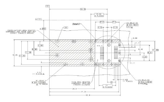
Datum and Basic Dimension Established by Customer Rads and Vias are Chassis Ground, 11 Places Through Holes are Unplated
