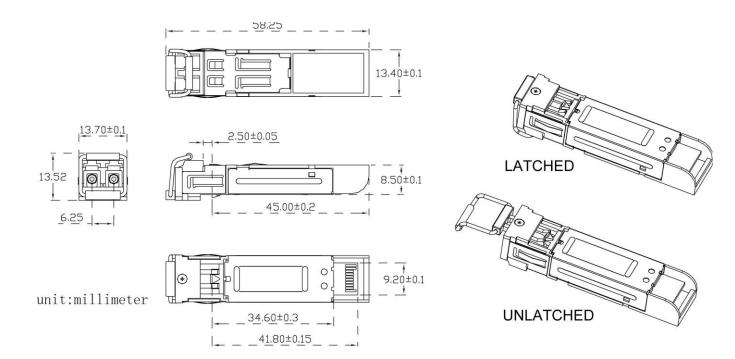
ALL DIMENSIONS ARE  $\pm 0.2 \text{mm}$  UNLESS OTHERWISE SPECIFIED UNIT: mm
