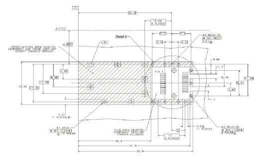
Detum and Basic Dimension Established by Customer Reads and Vias are Chassis Ground, 11 Places Chrough Holes are Unplated
