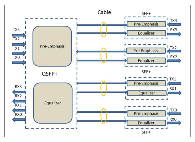
The transmitter side accepts electrical input signals. All input data signals are differential LVPECL or CML logic and they are internally terminated. The parallel input electrical signal first is processed via the Pre-Emphasis.
