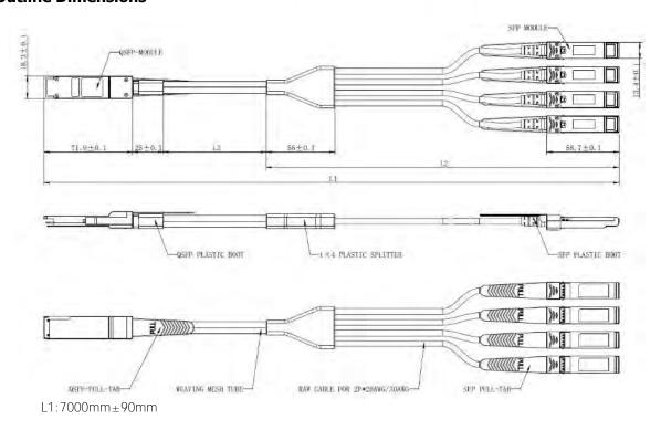
ALL DIMENSIONS (NOT INCLUDING THE LENGTH OF THE CABLE) ARE  $\pm 0.2 mm$  UNLESS OTHERWISE SPECIFIED UNIT: mm
