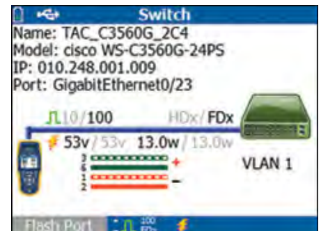
100 Mbps link on copper with PoE on port 23
