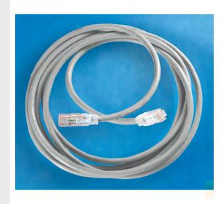
Clarity 6 Modular Patch Cord, gray, 15', Category 6, four-pair UTP stranded 24 AWG PVC/CM, center tuned with Clarity 6 connecting hardware for optimum Category 6 installed performance using Ortronics Paralign 2 pair-positioning technology
