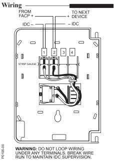
WARNING! Do not loop wiring under any terminals. Break wire run to maintain IDC supervision.
