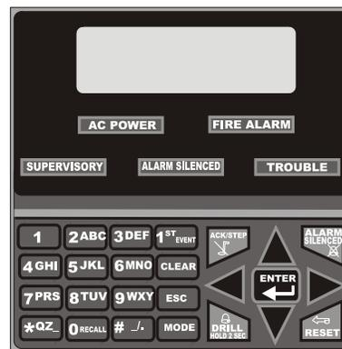
Figure 1.2 Membrane/Display Panel
