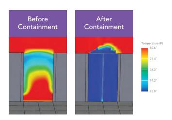
CFD analysis shows a significant reduction in hot air recirculation when Bi-Directional Doors are applied in conjunction with Rack Top Baffles at the end of the cold aisle.
