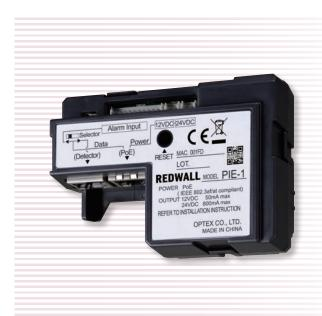
PIE-1 is an encoder that converts analog relay outputs to original ASCII code (Redwall Event Code) for Redwall and Fiber SenSys detectors. Detectors can be connected to Video Management Software platforms with PIE-1 and control IP cameras.
