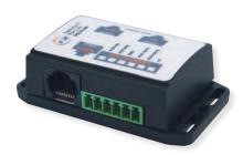
The TZ Centurion Port Link provides a connection for one TZ locking device plus RS485 and power connections for the continuation of the TZ network or connection of an additional TZ device (if it is being installed at the end of a network branch) and has I/O connectors for accessories like sensors, in-cabinet task lighting and fans.
