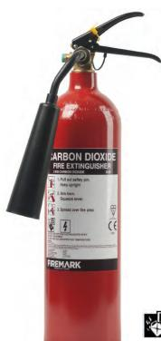
Carbon dioxide (CO,) extinguishers are suitable for fires involving flammable liquids and electrical hazards. The non-corrosive and non-conductive qualities of carbon dioxide make it an ideal choice for dealing with fires involving electrical equipment and machinery.
