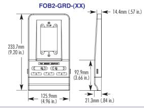
FOB2-(XX) .....Includes base, cover, designation labels, clear label covers, mounting hardware, cable ties, icons, and three blank bezels
