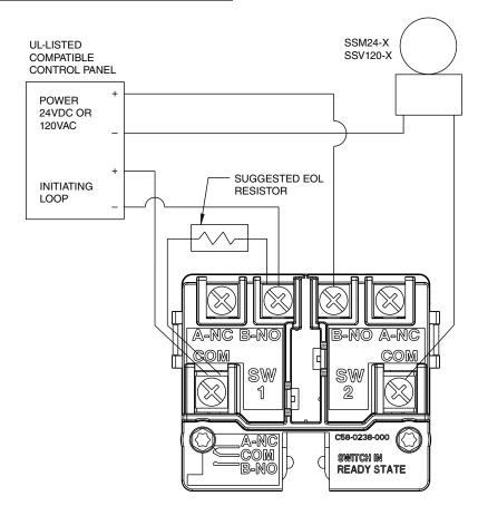
NOTE: COMMON AND B-NO CONNECTIONS WILL CLOSE WHEN VANE IS DEFLECTED, I.E., WHEN WATER IS FLOWING. DUAL SWITCHES PERMIT APPLICATIONS TO BE COMBINED ON A SINGLE DETECTOR.
