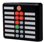
**RED** means all enclosure doors are closed and secure.
