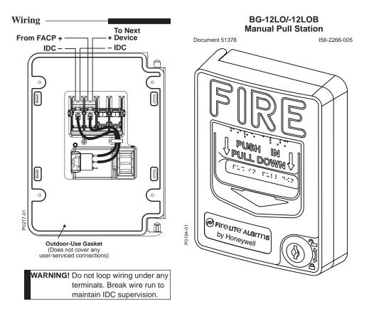
**CAUTION!** Do not detach the door of the pull station during installation. The door of the pull station cannot be reattached to the backplate after the backplate has already been installed onto an electrical box.
