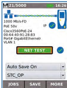
Press the Autotest button to display summary information and allow for detailed inspection of network parameters.
