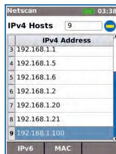
Display list of IP and MAC addresses of every device connected to the network.
