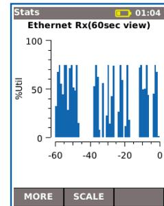
Real time display of broadcast network traffic shown as a percentage of port speed for the previous 60 minutes.
