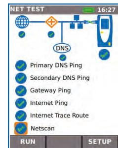
View network illustration to verify test results of each network component.
